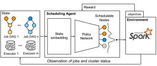
Figure 1: Clotho uses reinforcement learning (RL) to train an end-to-end system for a high-level objective. Its graph-based state embedding combines DAGs and feeds a policy network that makes the next scheduling decision.
