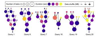
**Figure 2:** Data-parallel jobs have complex data-flow graphs like the ones shown (TPC-H queries in Spark), with each node having a distinct task duration distribution, number of tasks, and input/output size.
