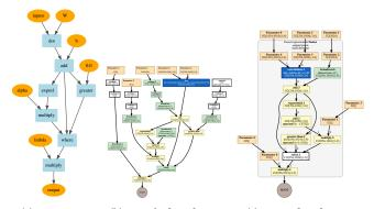
(a) JAX trace. (b) HLO before fusion. (c) HLO after fusion. Figure 1: XLA HLO fusion for a layer with SeLU nonlinearity. The gray box indicates all ops are fused into the GEMM.
