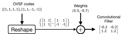
Figure 3: Filter generation process. Here we show an example of using two OVSF basis to generate a  $1 \times 2 \times 2 \times 1$  convolutional filter.
