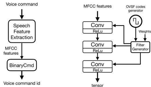
Figure 1: System architecture. Figure 2: BinaryCmd’s core.
