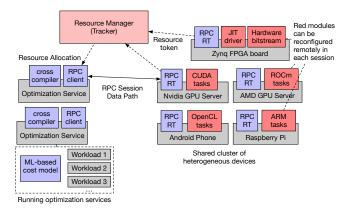
*Figure 1.* Overview of the TVM RPC system used by AutoTVM. AutoTVM optimization services request hardware resources from a centralized tracker that allows a wide range of hardware devices to be shared across optimization tasks. This system allows optimization algorithms to use arbitrary hardware devices, regardless of the algorithm's compute platform.
