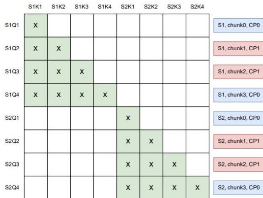
Figure 1. Load-balanced CP sharding with fused inputs in full prefill with 2 CP ranks (CP2). We have 2 input sequences: S_1 , S_2 . Each is partitioned evenly into 4 chunks: Q_i / K_i , where i = 1, 2, 3, 4 .
