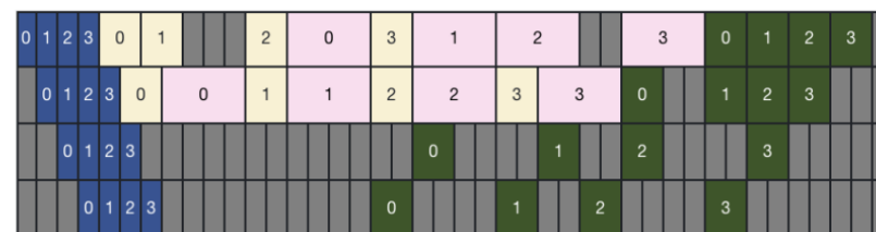
(b) Pipeline when PP degree is 4 (default No-Op insertion).
