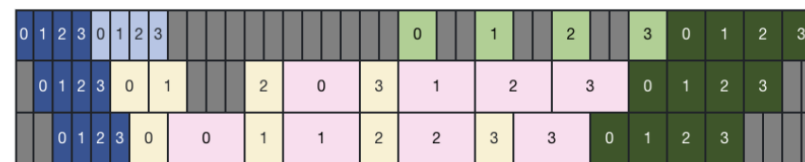
(a) Pipeline when PP degree is 3.
